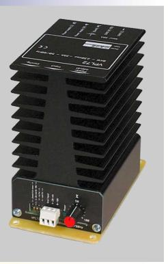
Power controller with analog command. The output modulation can be phase angle variation or burst fired (zero -cross), allows extremely fine and fast modulation of resistive loads even with low thermal inertia as infrared.
